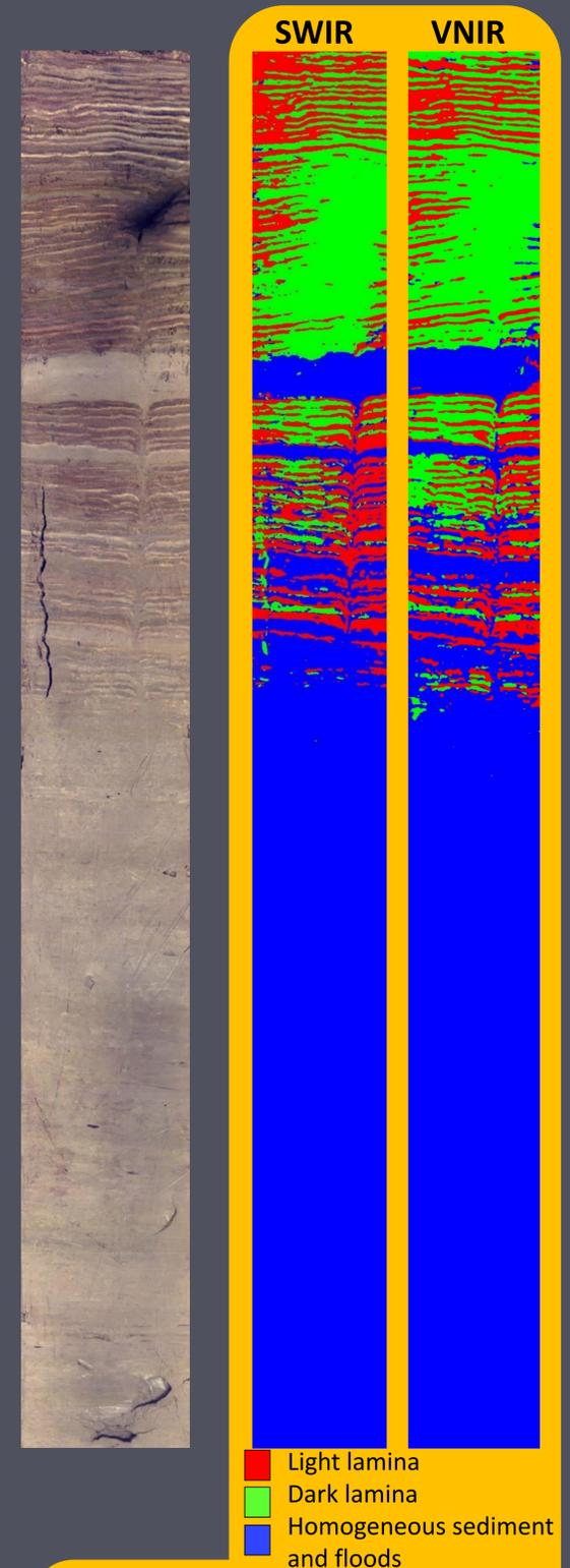
Accuracy of the 2 camera lithology classification models are 97.3% (SWIR) and 98.4% (VNIR). Then, it is possible to estimate the number of lamina : 136 $\pm$ 2 (SWIR), 140 $\pm$ 2 (VNIR), with eye counting it is 134 $\pm$ 5.
