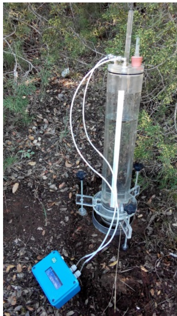
Fig. 3. Compact automated infiltrometer proposed by Di Prima (2015). The device consists of a containment ring with a small head of water that is controlled by a Mariotte reservoir and a data acquisition system based on the open source microcontroller platform Arduino.
