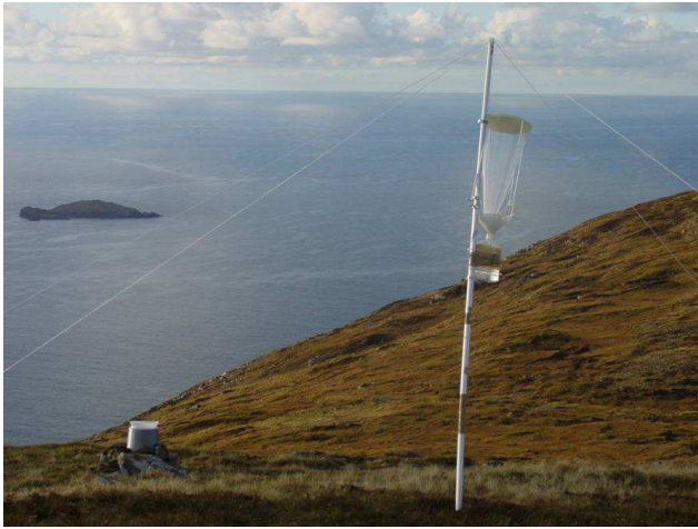
Fig. 1. Cloud collector set up on Caepabhal. Collector was erected onto the end of a 2 m pole and secured with guy ropes.
