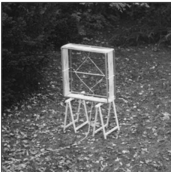
Fig 7: 137kHz receiving loop antenna.
