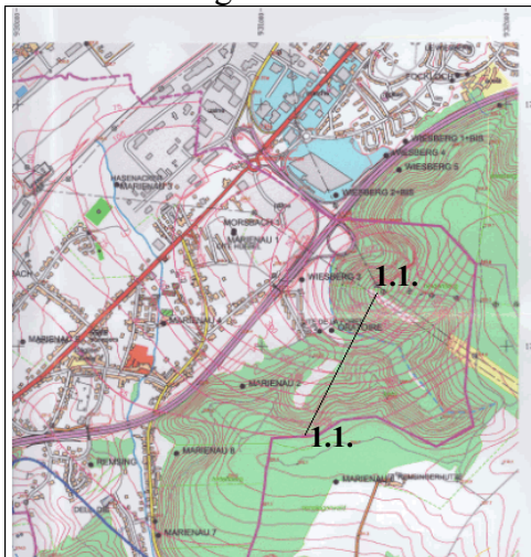
Figure 6: Final subsidence and location of cut A-B
