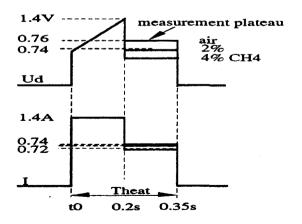
When  $Rd(T) = 1.03 \Omega$ , the controller reduces intensity in order to maintain Rd at this value.
