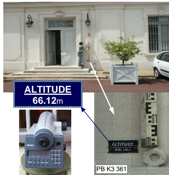
Figure 3.2.1 The NGF leveling point on the wall of the Observatoire building of BIPM and its value 66.12m in the NGF served as the starting value of the height measurement before the RGC2009. The same point in the new IGN system is numbered P.B.K3-361 with its value 66.4558m in IGN69. The difference between the two systems is: \text{IGN69-NGF}=+0.3358\text{m} . The levelling instrument used by IGN was the Zeiss Dini 10
