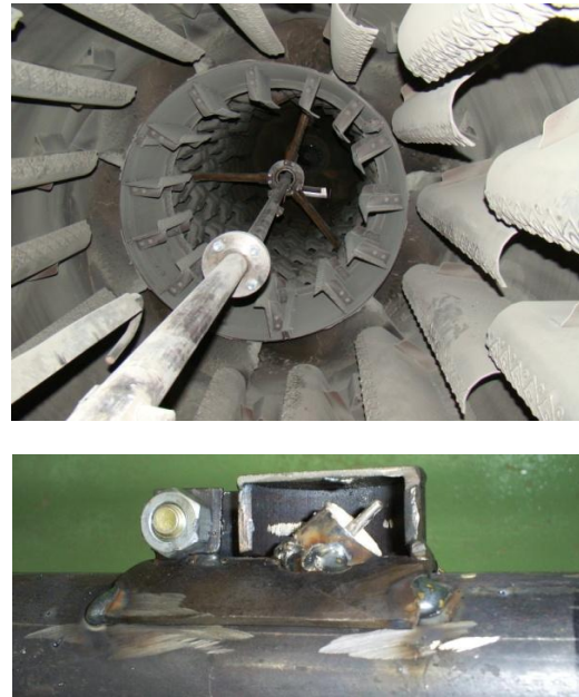
Fig. 9. probes support in the rotary drum and probe
