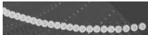
FIGURE 2: Typical sequence showing the spinning motion of a spherical particle onto the rotating plate.
