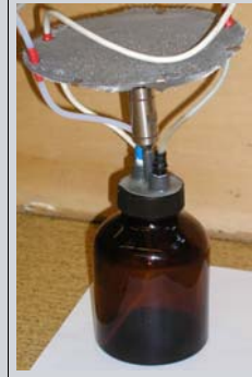
Sampling bottle, valve and "area lysimeter"
