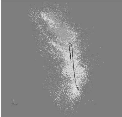
Fig.1: Plan view of the locations of the generated events at Soultz after the hydraulic stimulation of GPK2 borehole (top trace), GPK3 borehole, and GPK4 borehole (bottom trace)
