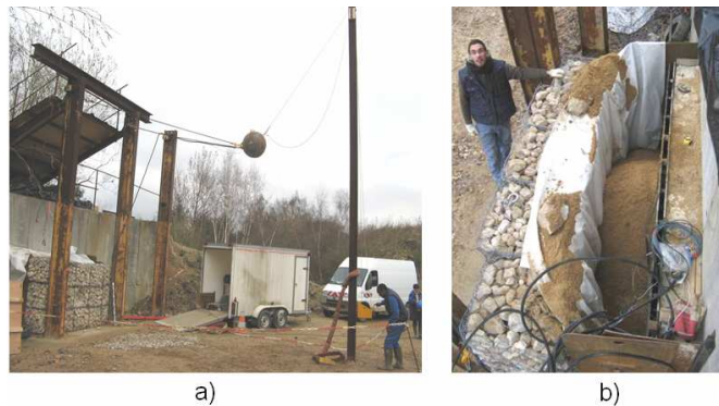
Figure.2. Overview of the experimental device (a) and the impacted structure during the implementation (b).
