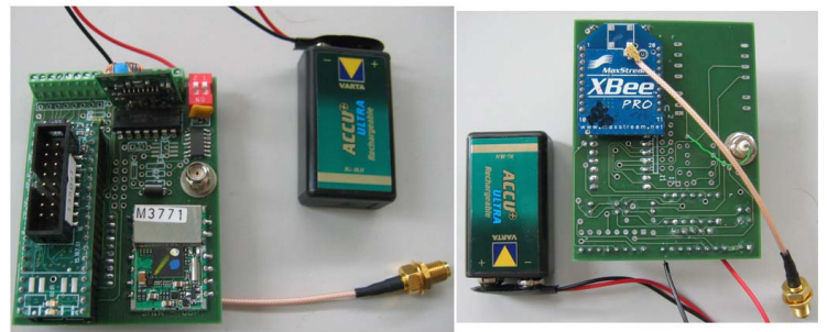
Fig. 5. LiveNCM gateway design
