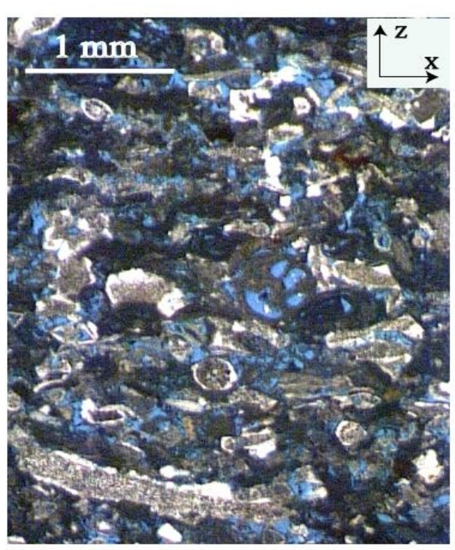
Figure 1. Thin section of Meriel limestone. The porous network is represented by blue epoxy.
