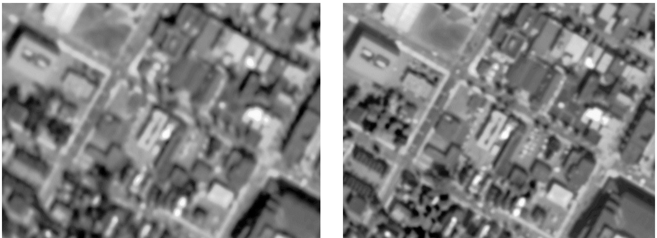
Figure 5: Quickbird image of Fredrickton, Canada. Red modality, resolution 2.8 m. On the left, original image, copyright DigitalGlobe 2002. On the right, fused image.
